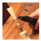
**12.** REMOVE MANDREL #3 AND PRESS THE REED BLANK TIGHLY ONTO THE PIN ON THE DRYING RACK TO DRY FOR AT LEAST 3 DAYS.
