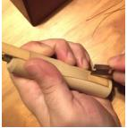
4. FOLD THE CANE OVER A KNIFE AT THE CENTER LINE OF THE CANE
